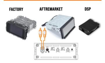
The RZA500.2 is designed to accept any analog audio signal from an aftermarket, factory radio, or DSP.
